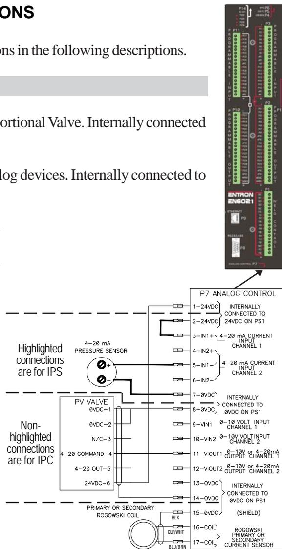
**Figure 1-10. P7 connections**
