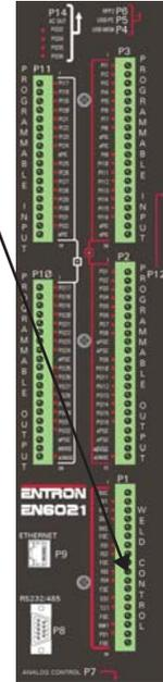
\* These inputs must be jumpered out if not used.
