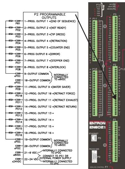
Figure 1-7. P2 connections
