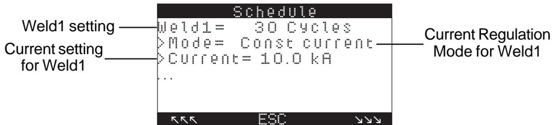
Figure 5-27. *WELD1 in Constant Current mode*
