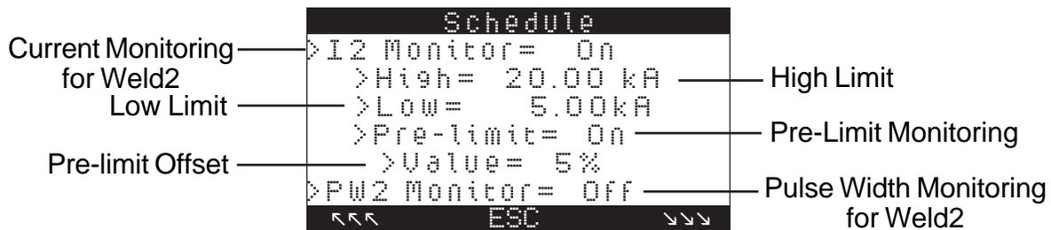
Figure 5-32. CURRENT MONITORING for WELD2
