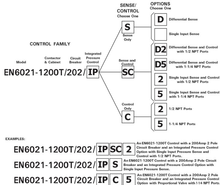
Figure 9-58. IPSC configurations
