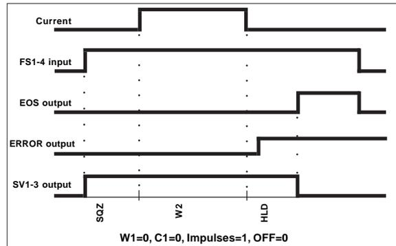
**Figure 9-2.** Basic Spot Weld—Weld Fault
