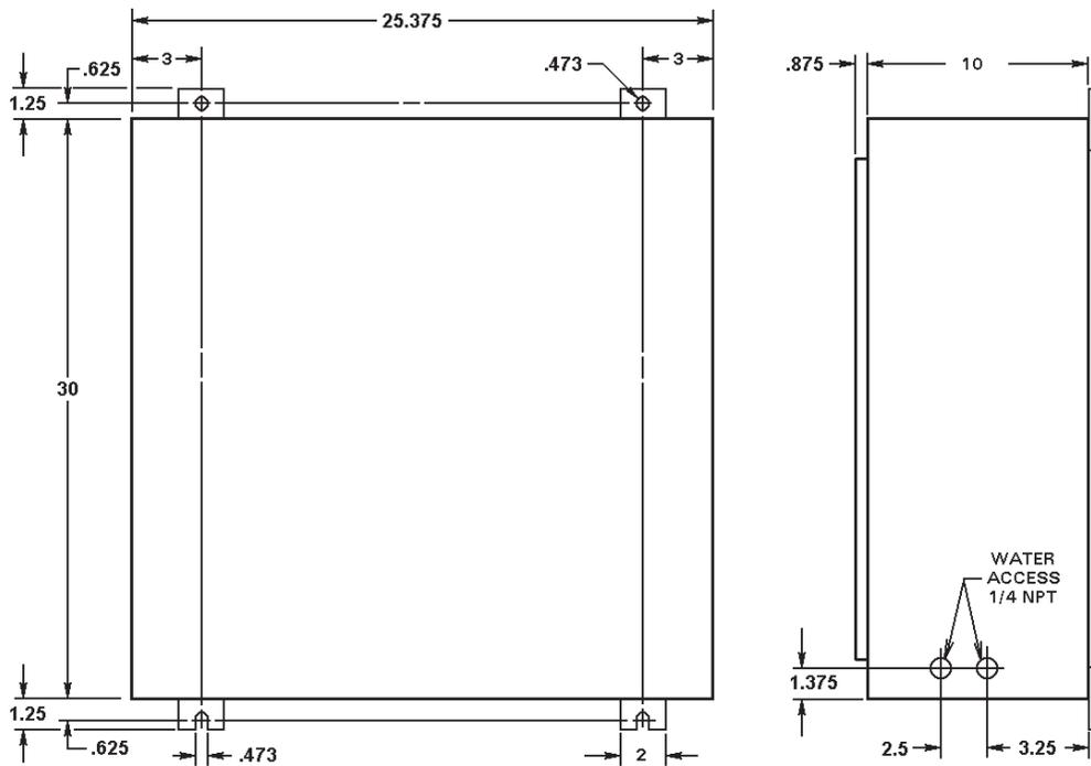
**Figure 2-4.** Mechanical mounting diagram for “N” Cabinet
