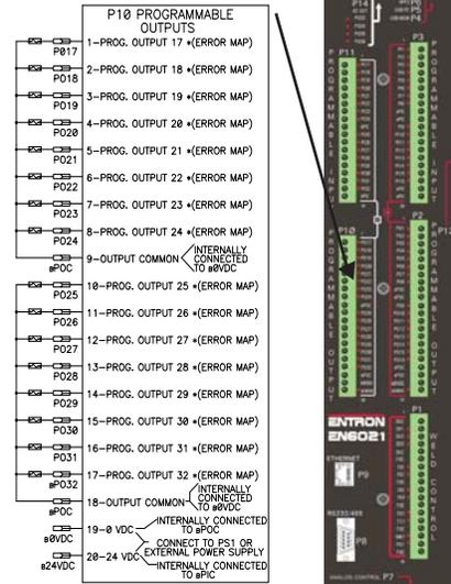
Figure 1-14. P10 connections
