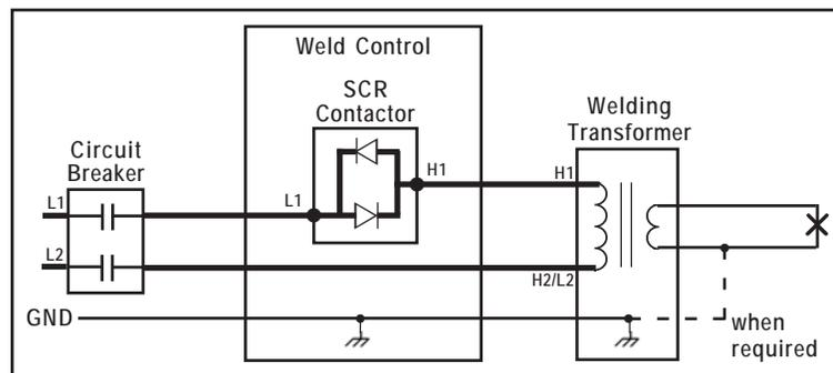
Figure 4-6. Power connections
