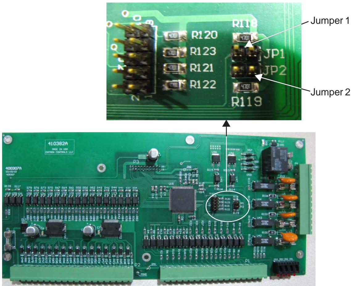
**Figure 1-16.** Installation of I/O Expansion Card Jumpers (P/N 331139)
