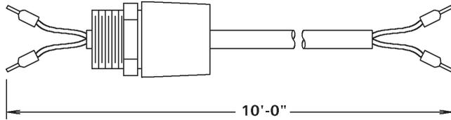
Operating Temperature:  $-22^{\circ}\text{C}$  to  $80^{\circ}\text{C}$  ( $0^{\circ}\text{F}$  to  $175^{\circ}\text{F}$ )
