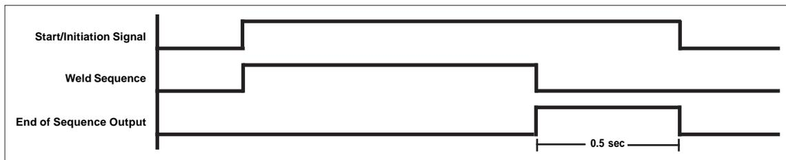
**Figure 9-3.** End of Sequence in Spot operation
