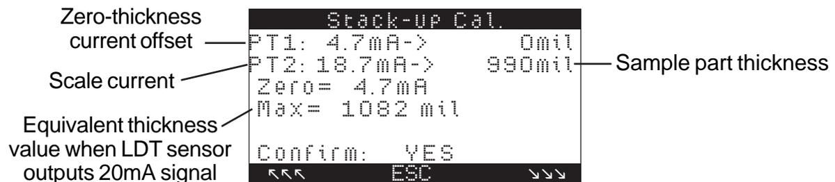
Figure 5-55. Stack-up Calibration sub-menu
