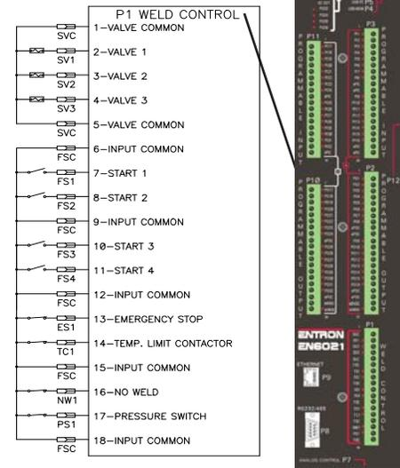
**Figure 1-6.** P1 connections
