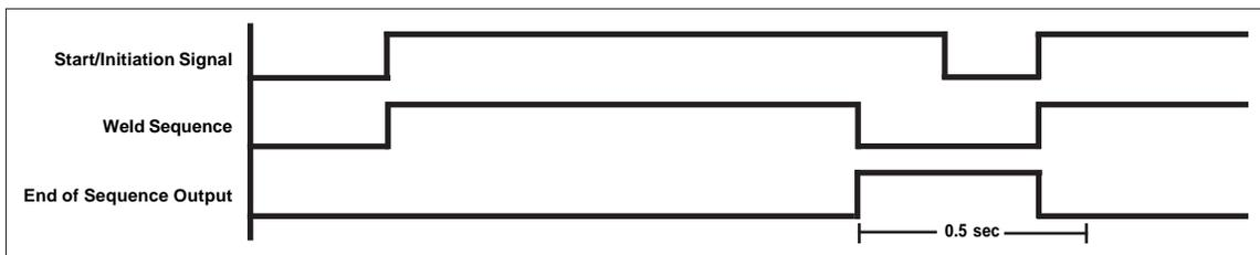
**Figure 9-4.** End of Sequence with new start/initiation signal
