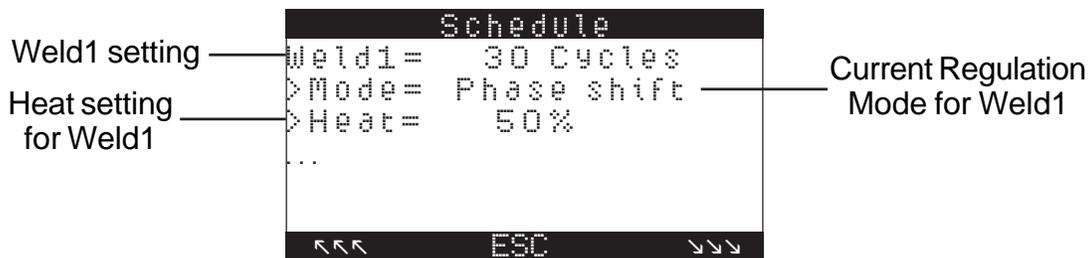
Figure 5-26. *WELD1 in Phase Shift mode*
