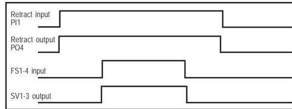
Figure 9-29. Maintained Retraction
