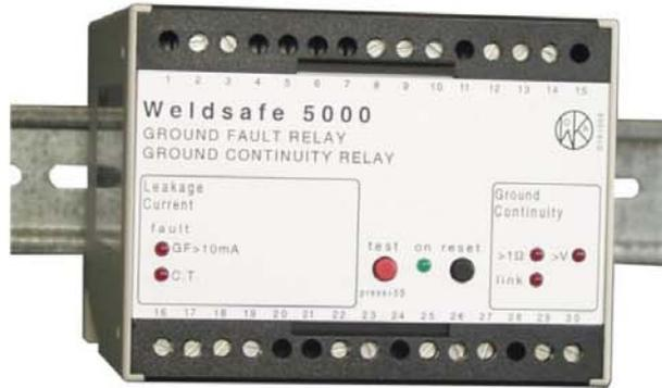
The Weldsafe 5000 combination ground fault current and ground check relay has been designed to provide sensitive ground fault protection and continuous ground checking for ac, 50-60 Hz manual transguns in accordance with RWMA Bulletin 5 standards.
