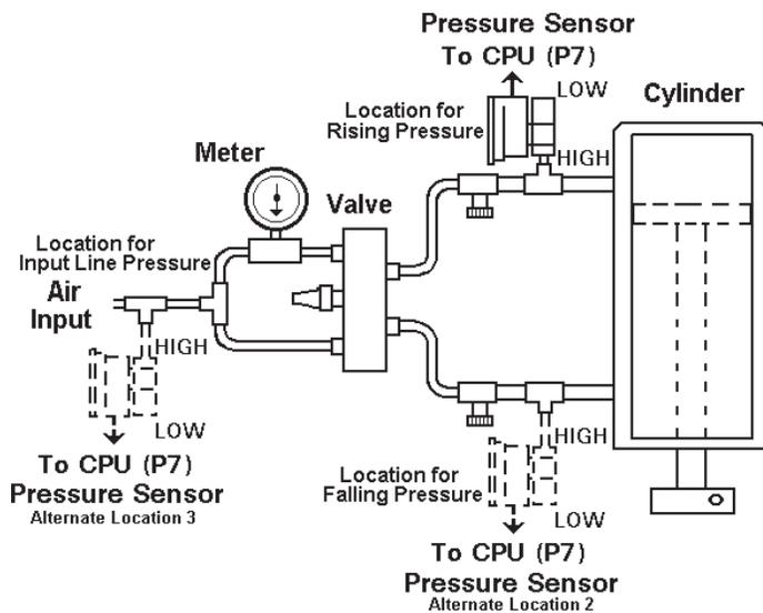
**Figure 9-64.** *IPS System with Differential Pressure Sensor*
