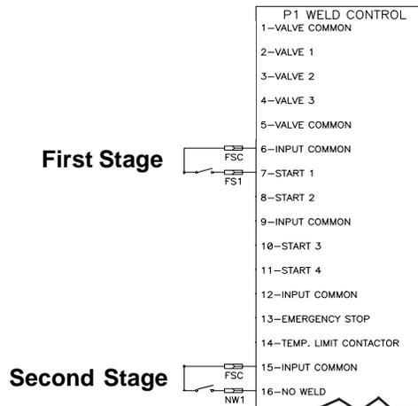
**Figure 9-25.** Two Stage initiation in Brazing mode
