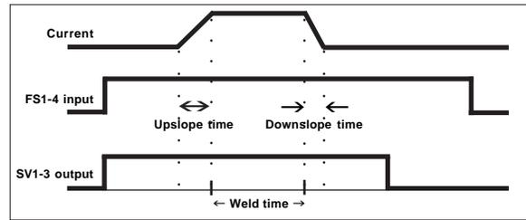
Figure 9-10. SLOPE function in Spot Weld
