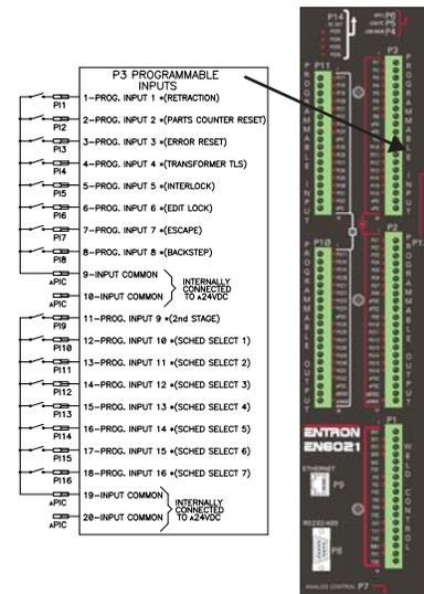
**Figure 1-8.** P3 connections
