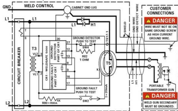
Typical Diagram. For details see Wiring Diagram
