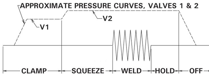
**Figure 9-14.** *Butt Weld with Chained CYCLE MODE*
