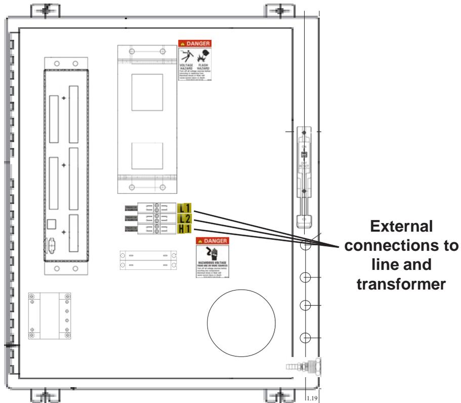
Figure 4-7. Wiring Diagram for External SCR Contactor
