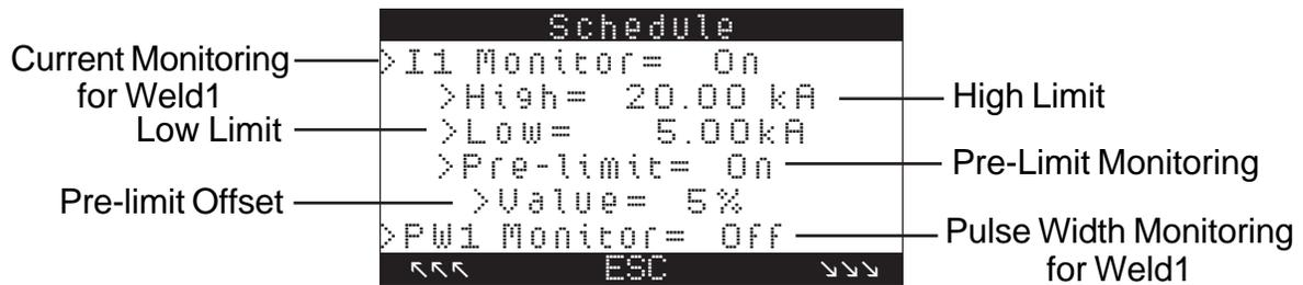
Figure 5-28. CURRENT MONITORING for WELD1
