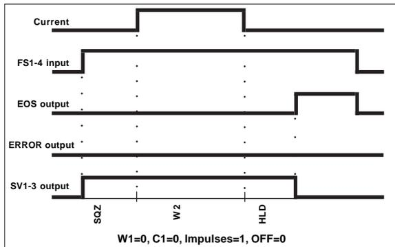
**Figure 9-1.** Basic Spot Weld—No Weld Faults
