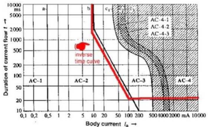
Weldsafe 5000 Ground Fault Setting 2 reaction time
