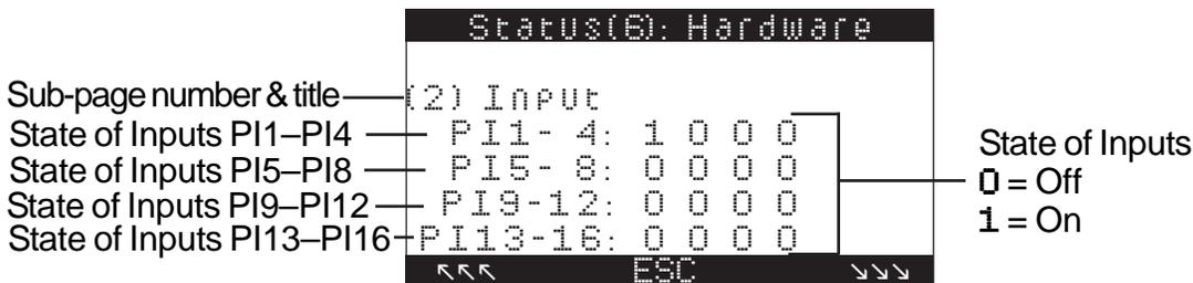
**Figure 5-13. Hardware Inputs**
