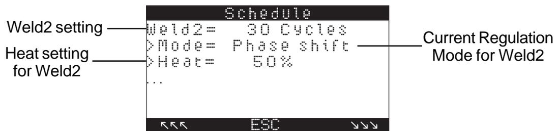
Figure 5-30. *WELD2 in Phase Shift mode*
