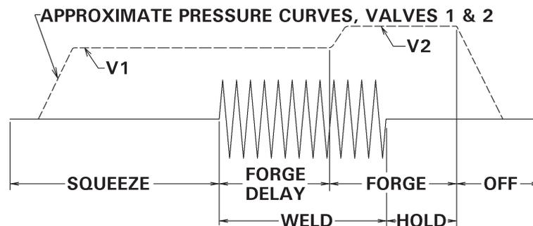
**Figure 9-15.** Forge Delay with Chained CYCLE MODE
