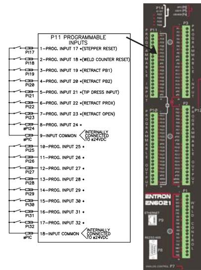
Figure 1-15. P11 connections
