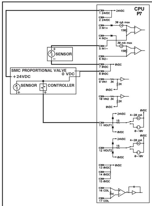
**Figure 9-67.** IPSC Wiring Logic –
