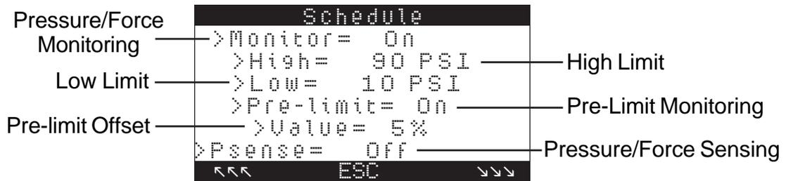
**Figure 5-23. PRESSURE/FORCE MONITORING**
