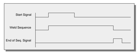
In Repeat Spot operation the End of Sequence output switches on for the Off time between sequences, and momentarily after the final sequence.
