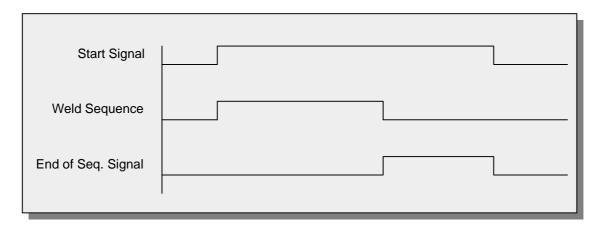
In Single Spot operation, at the end of the weld sequence the End of Sequence output switches on. If the Start signal is absent, the End of Sequence signal switches on only momentarily.
