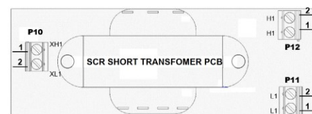
Figure 11 transformer PCB wiring
